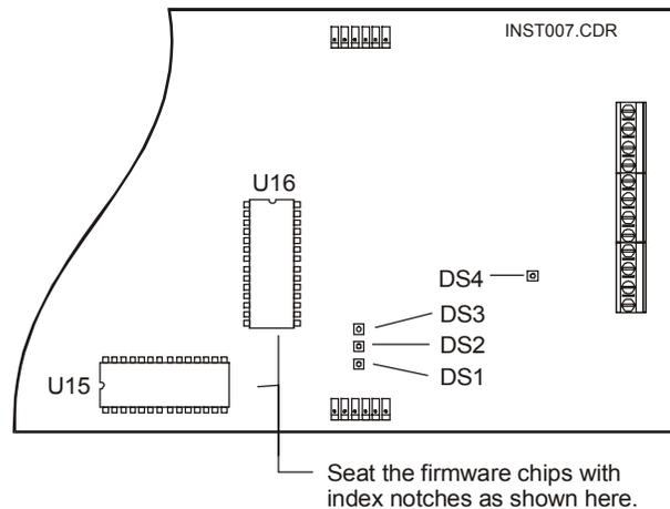
Figure 4-8: Main Controller Module
