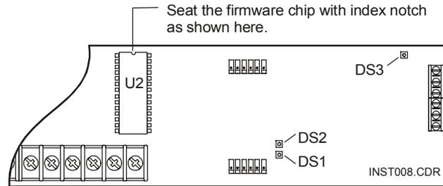
Figure 4-9: Expander Loop Module
