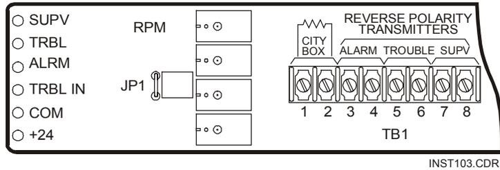
Figure 3-1: Reverse Polarity Module
