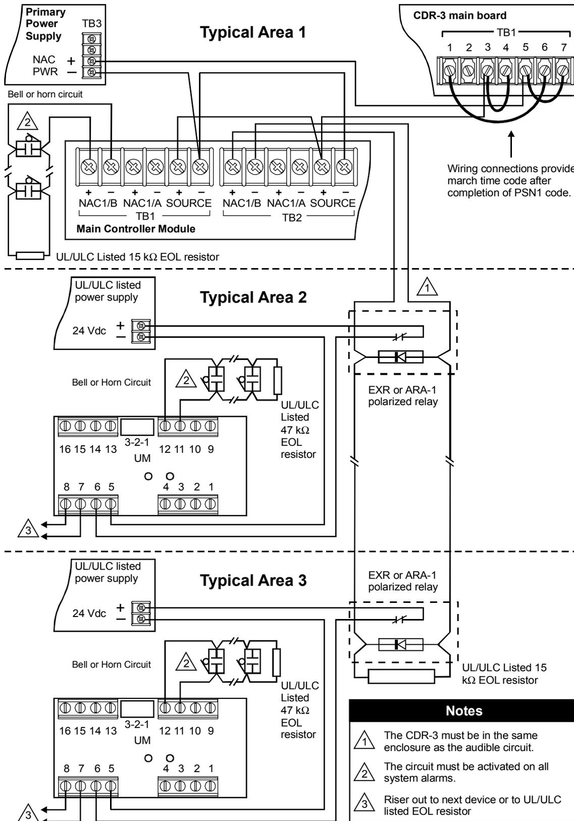
Figure C-5: Coded NAC risers
