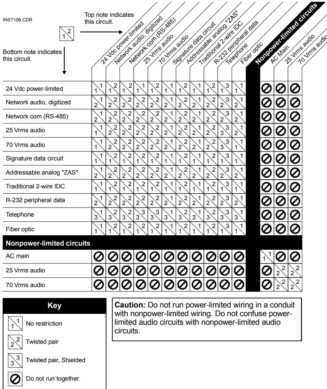
Figure A-1: Circuit compatibility matrix
