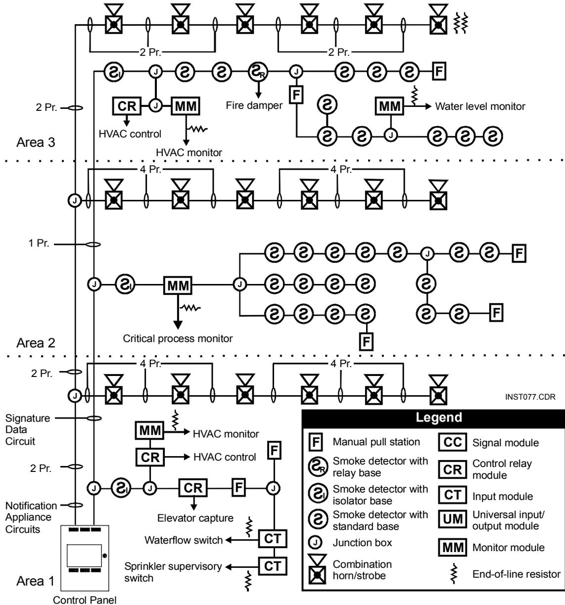
Figure 2-5: Typical Class B NAC wiring
