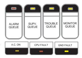
queue have been reviewed using the Alarm Queue button. Since all alarms are latched until the panel is reset, the LED will remain on until then.
