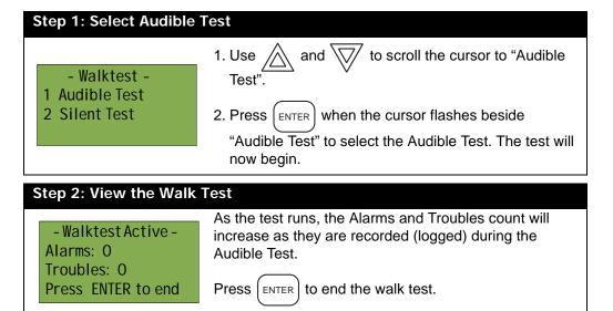
At this point the display will vary, depending on whether or not a printer is connected to the panel. **If a printer is not connected to the panel**, the walk test will print to the display.
