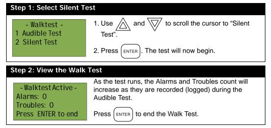
At this point the display will vary, depending on whether or not a printer is connected to the panel. **If a printer is not connected to the panel**, the walk test will print to the display.
