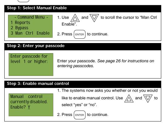
The display will now show the message "Manual control enabled" while in normal mode, and the panel will be in a trouble condition. To check which annunciator manual control was enabled on,
