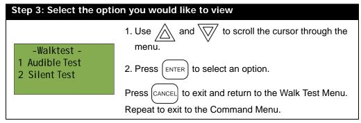
The subsections below provide instructions on using each Walk Test Menu option.
