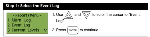
At this point the display will vary, depending on whether or not a printer is connected to the panel. **If a printer is not connected to the panel**, the Event Log will print to the display.
