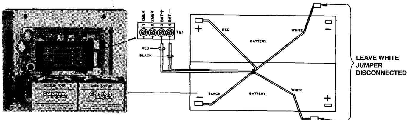
**NOTE:** IF BATTERIES ARE IN EXTERNAL CABINET, ROUTE HARNESS THROUGH KNOCKOUT CLOSEST TO CONTROL PANEL.
